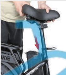
Insert the seat tube according to the direction and adjust the height
