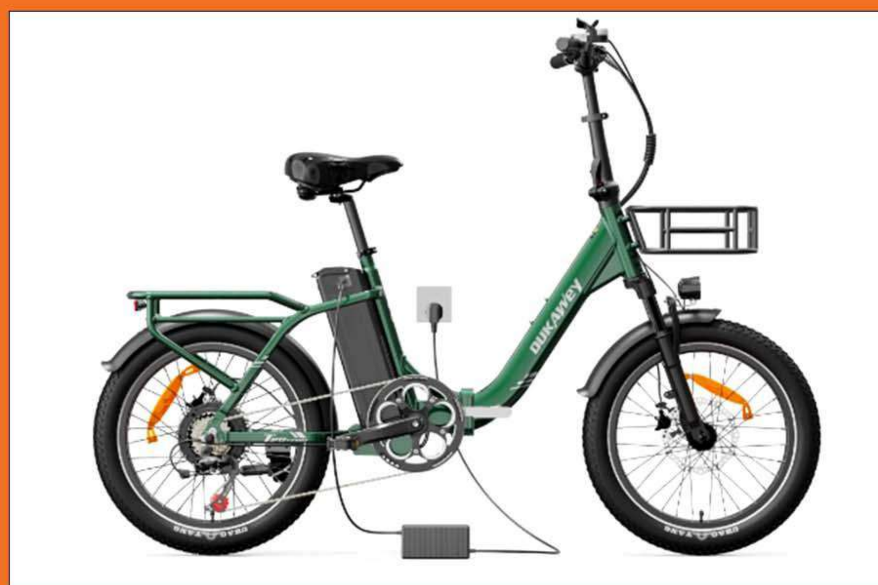
A. Recharge the battery on E-Bike directly
