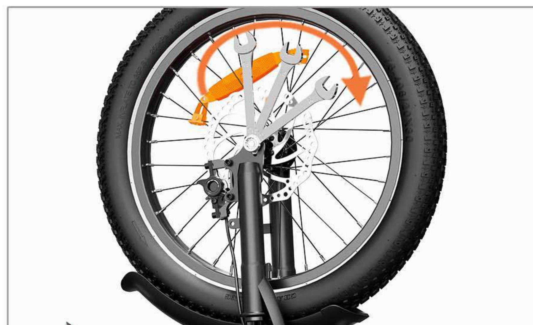
11 Use the tool to tighten the large nut After the front wheel installation is completed, flip the vehicle back over
